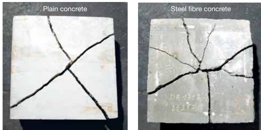
Fig. 2: The crack pattern observed on the plate test
